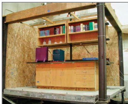
Shake table test at UC Irvine includes non-structural elements (photo: PEER Testbed Study).
